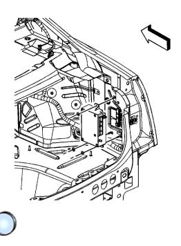
Important: The vehicle communication interface module (VCIM) has a specific set of unique numbers that tie the module to each vehicle. These numbers, the 10-digit station identification (STID) and the 11-digit electronic serial number (ESN), are used by the National Cellular Network and OnStar® to identify the specific vehicle. Because these numbers are tied to the vehicle identification number of the vehicle, you must never exchange these parts with those of another vehicle.
